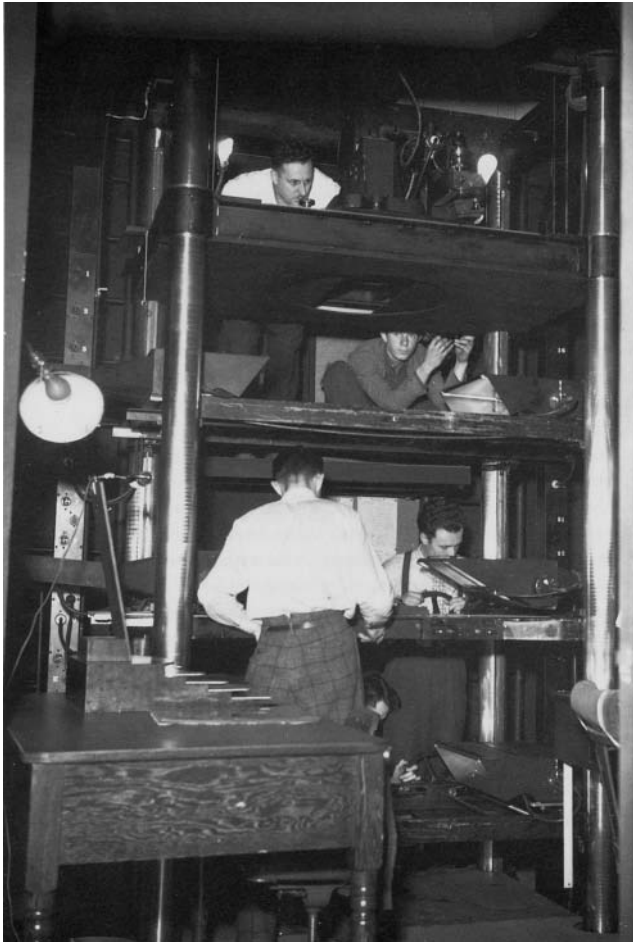
Figure 1.3 Disney multiplane camera
