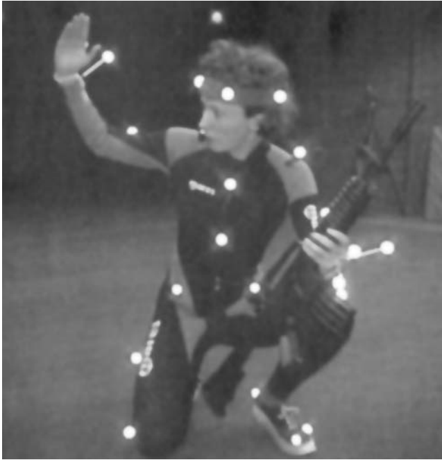
Figure 6.50 Image from optical motion capture session [20]
