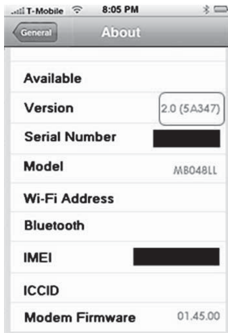
Figure 3-7 The iPhone's version number can be seen on its About screen.
