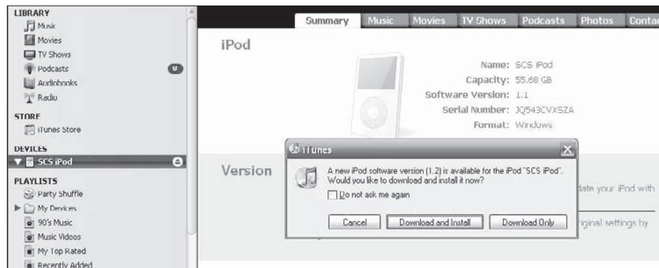
Figure 3-6 Connect an iPod to iTunes to view the firmware version.
