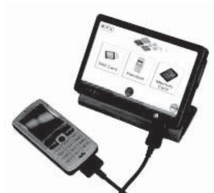
Figure 3-26 Aceso downloads data stored in SIM cards and memory cards directly from the phone.
