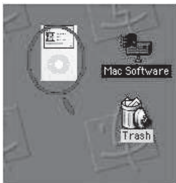
Figure 3-2 Drag the iPod icon to the Trash to unmount it.
