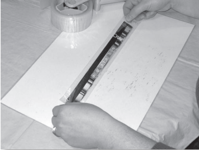
Laminating the paper strip by covering it with packing tape
