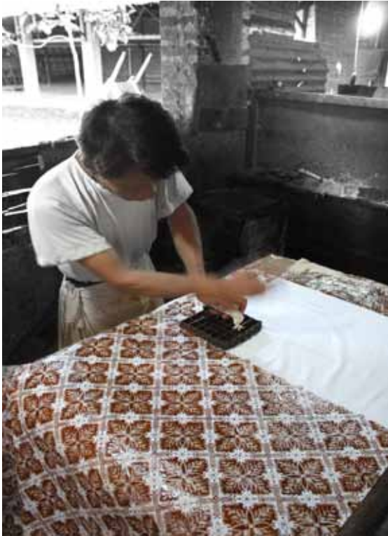
The making of "batik cap." In this method, hot malam or wax is applied on cloth surface using a specially constructed metal stamp, usually from copper.
