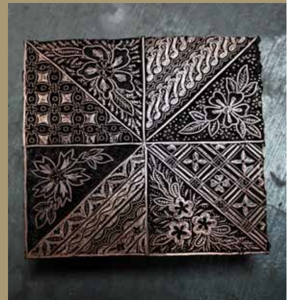
Stamping is a way to produce high quality batik in higher volume. The stamps are made from thin copper sheets, arranged and constructed accordingly to create the desired designs.
