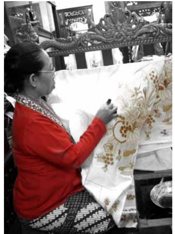
A woman applies wax using canting . Various designs are created by using different size of canting.
